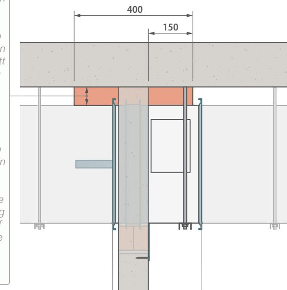
Provide appropriate break-away / flexible joint between fire damper and connecting ductwork on both sides of the assembly tunnel.
